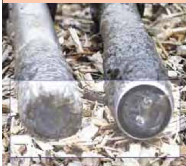
Sensor without and with ultrasound cleaning system after 30 days
